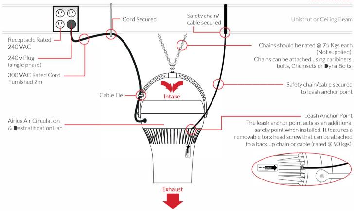
NOTE: Do not hard connect any Airius model 60 fans to structure - use chain (preferred) or cable only
